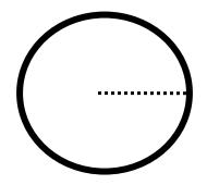
Radius – a straight line extending from the center of a circle to its edge.
